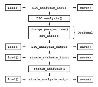
The first step for performing DIC is to form a DIC analysis input:
